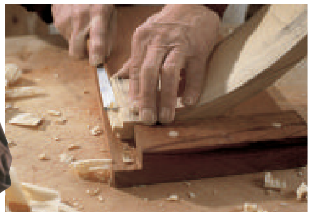
The author used a backsaw to cut the tenons for this table. Then he turned to his chisels to pare the tenons, creating a slight angle to accommodate the curved aprons.
