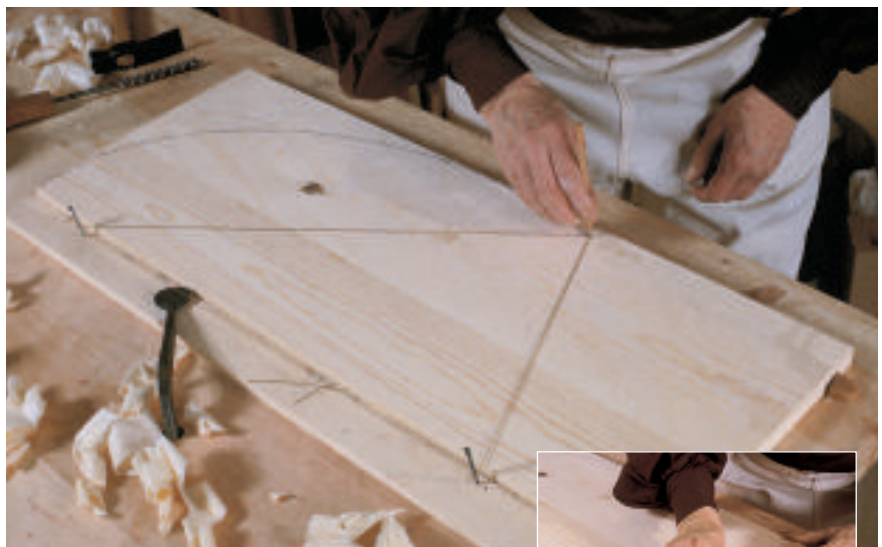
The old "two-nails-and-a-string" method is a time-honored way to lay out a perfect ellipse. Shorten the string and move the nails to draw the apron locations.
