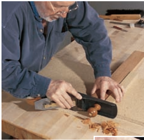
A shooting board gives you a clear view of the cut as you progress toward the knife line.
