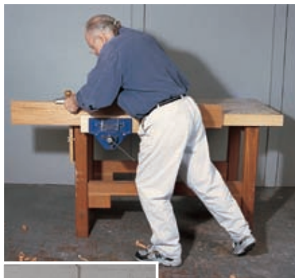
Begin the stroke with all your weight on your rear foot (left), then transfer your weight as you propel the plane forward (above).
