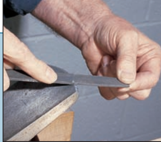
File a substantial chamfer on the toe and heel of the plane.
