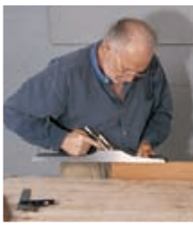
The plane gets its power from your legs and feet. You can plane about 5 feet of wood without having to travel.
