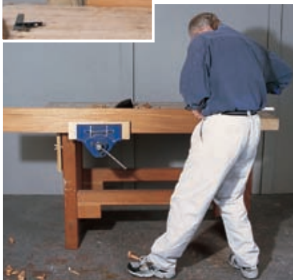
The plane gets its power from your legs and feet. You can plane about 5 feet of wood without having to travel.
