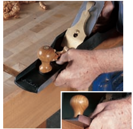
To plane a narrow edge, grip the toe of the plane between your thumb and fingers. By touching the workpiece, your fingers act as a fence. Look down into the plane to monitor the progress of the cut.
