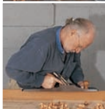
Begin the stroke with all your weight on your rear foot (left), then transfer your weight as you propel the plane forward (above).
