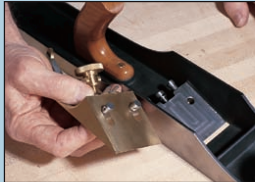
The bedrock style frog (above) firmly and ingeniously connects the blade assembly to the body. A regular frog is not as massive and does not seat as firmly.
