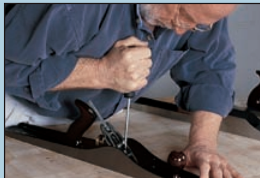
Adjust the frog to support the blade securely. The mouth opening should be set to 1/32".
