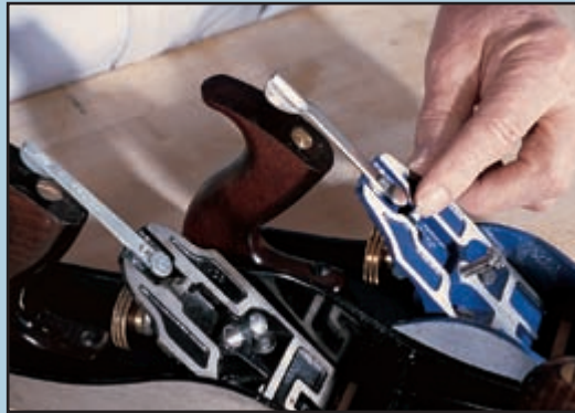
Old-style blade controls (left) are more robust than the stamped metal ones in recent planes.
