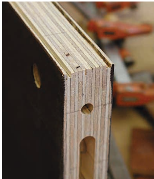
A pair of shallow relief grooves (formed on the table saw using a standard blade) prevent glue from squeezing out when installing the rail caps.
