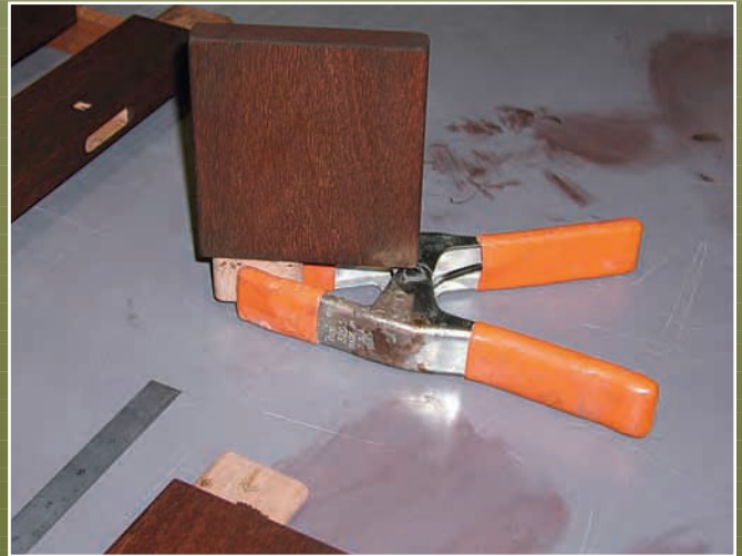
Slip a loose tenon into the short rail mortises so you'll have something to hold onto during staining. A spring clamp works well to hold these rails vertically while they dry.
