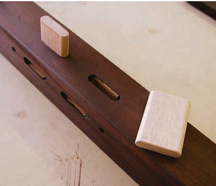
All of the leg and rail joints on this bedframe are assembled with loose tenons. The author makes them "production style" in long strips, then cuts them to length.
